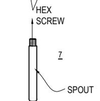
8. PLACE COLD AND HOT WATER HANDLES TO THE FAUCET AND TIGHTEN THE HEX SCREW.
