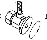
1. SHUT OFF WATER SUPPLY. REMOVE THE OLD FAUCET AND FLEXIBLE HOSES. CLEAN SINK SURFACE IN PREPARATION FOR THE NEW FAUCET.
