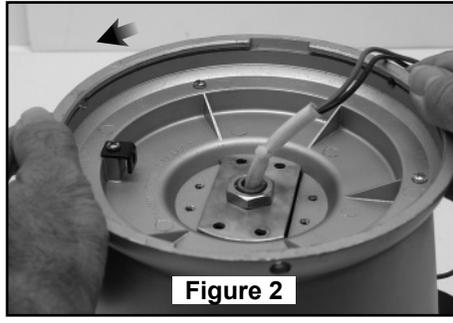
Fig 2. Remove the motor housing by rotating the housing so that the opening matches the flange.
