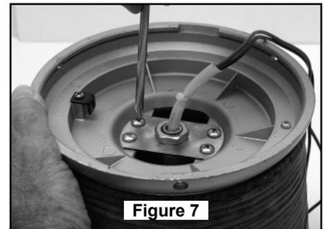
Fig 7. Assemble and tighten 4 screws.
