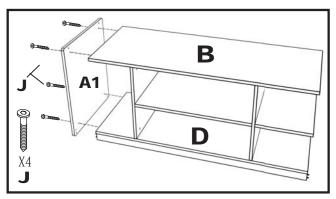
4A. Attach Left Side Panel(A1) to the assembled unit using 4 Flat Hex Screws(J). Tighten with the Hex Key Tool(K).
