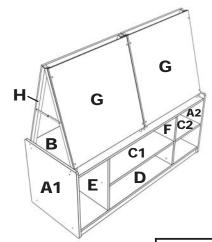
TIP! DO NOT FULLY **TIGHTEN SCREWS UNTIL ALL SCREWS** HAVE BEEN LOOSELY POSITIONED
