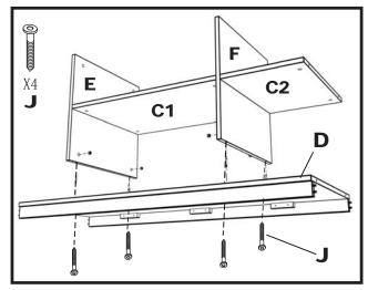
2. On a carpet or protected surface, attach Divider Section(C1,C2,E,F) to Bottom Panel(D) using 4 Flat Hex Screws(J). Tighten with the Hex Key Tool(K).
