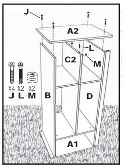
4B. Using 2 adults, turn the unit onto its Left Side(A1) on a carpet or protected surface, as shown. Insert 2 Metal Dowels(L) into the plastic plugs located inside the Right Side Panel(A2). Tighten with a Phillips Head Screwdriver.
