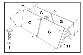
5. Attach the 4 Easel Boards(G) to the 4 Easel Frames(H) using 16 Round Hex Screws(I), using 4 in each Easel Board(G) as shown. Tighten with the Hex Key Tool(K).
