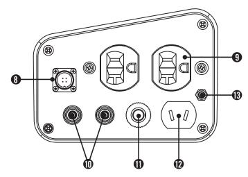
\* These outlets are used for connecting two Champion model 73536i generators for parallel operation. A Champion model 73500i cable kit (optional equipment) is required for parallel operation.
