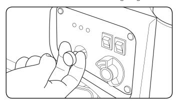
6. Turn the engine switch to the "On" position.
