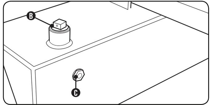
9. Unscrew and remove the tank fill plug, on top of the tank. Using a funnel add approximately 7 gal. (26.5 L) of hydraulic oil to the tank. Wipe up any spilled oil. (B)
