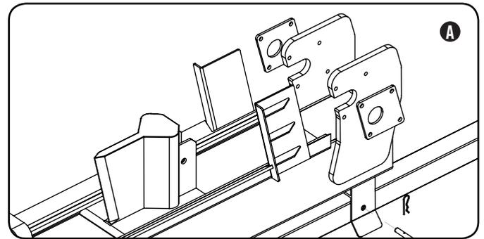
3. Install the cylinder by sliding the pegs at the end of the cylinder into the mounting slots on top of the beam. Be sure to slide the cylinder all the way back into the mounting slots. (B)
