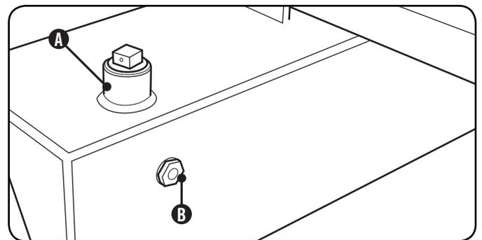
6. Start Engine. Extend and retract the wedge to purge air from the hydraulic system. When the wedge motion is smooth, the system is properly purged.
