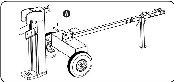
2. Slowly lift the front of the tow bar to roll the frame toward the beam and carefully align the pivot holes on the bottom of the beam and the top of the hydraulic oil tank.
