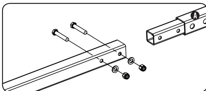
2. Attach the tow bar to the bracket on top of the hydraulic oil tank with two M12x85 bolts and M12 lock nuts. (B) Tighten to 50 ft-lb.
