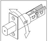
b. Insert deadbolt into edge of door. Install with two #8 x 3/4" flat head combination screws provided (see diagram for proper positioning). Ensure bolthead is extended throughout installation procedure.
