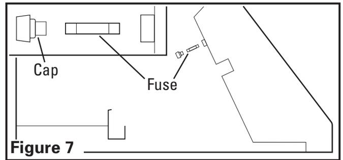
**NOTE:** If you need to replace the fuse, replace with a 1/4" x 1-1/4" Bussman MDA-10 or equivalent 10 amp, 250V ceramic, time delay fuse only.
