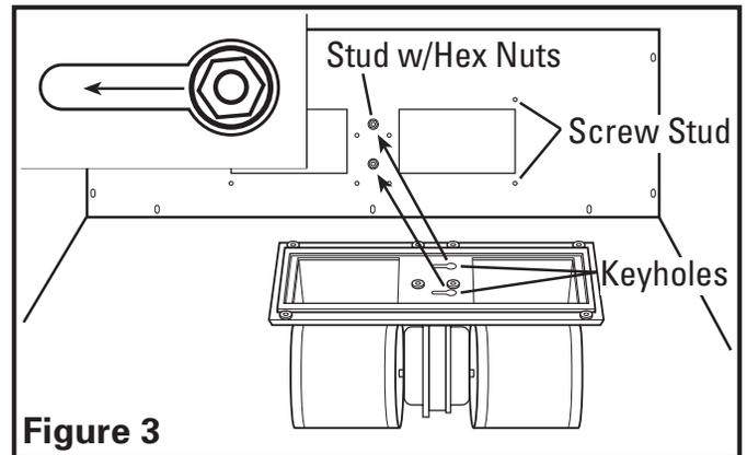
4. Using 8 of the included 8-32 screws and washers, mount the blower in place and tighten all screws. Confirm that the blower is securely seated in place and there are no air gaps around the blower gasket.
