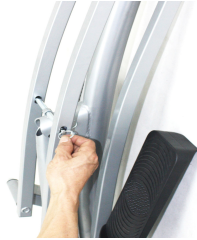
Remove the pin (part 10)
