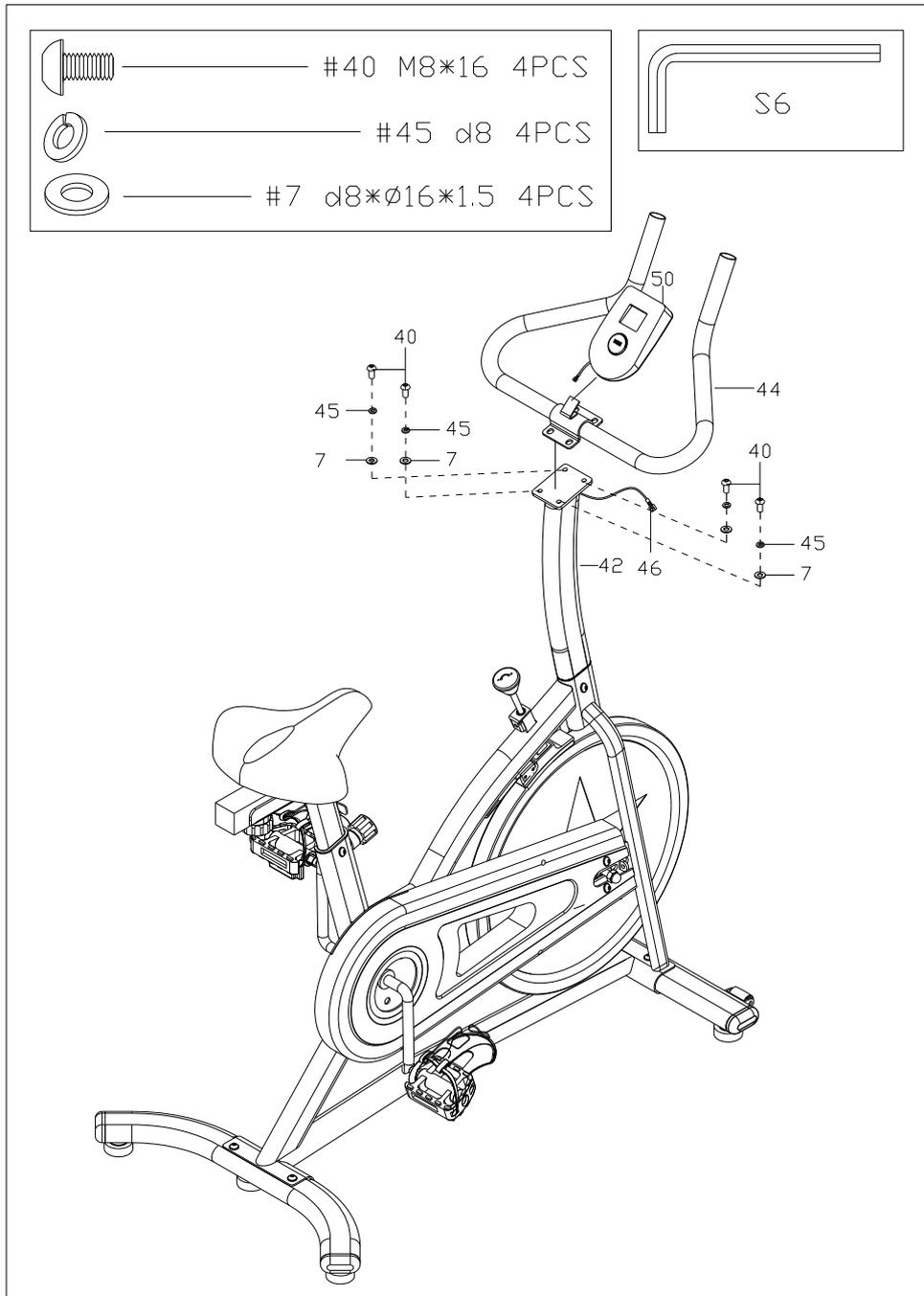
A. Assemble the Handlebar (44) on the Front post (42), and fix it with Screws (40), Spring washers (45) and Washers (7).
