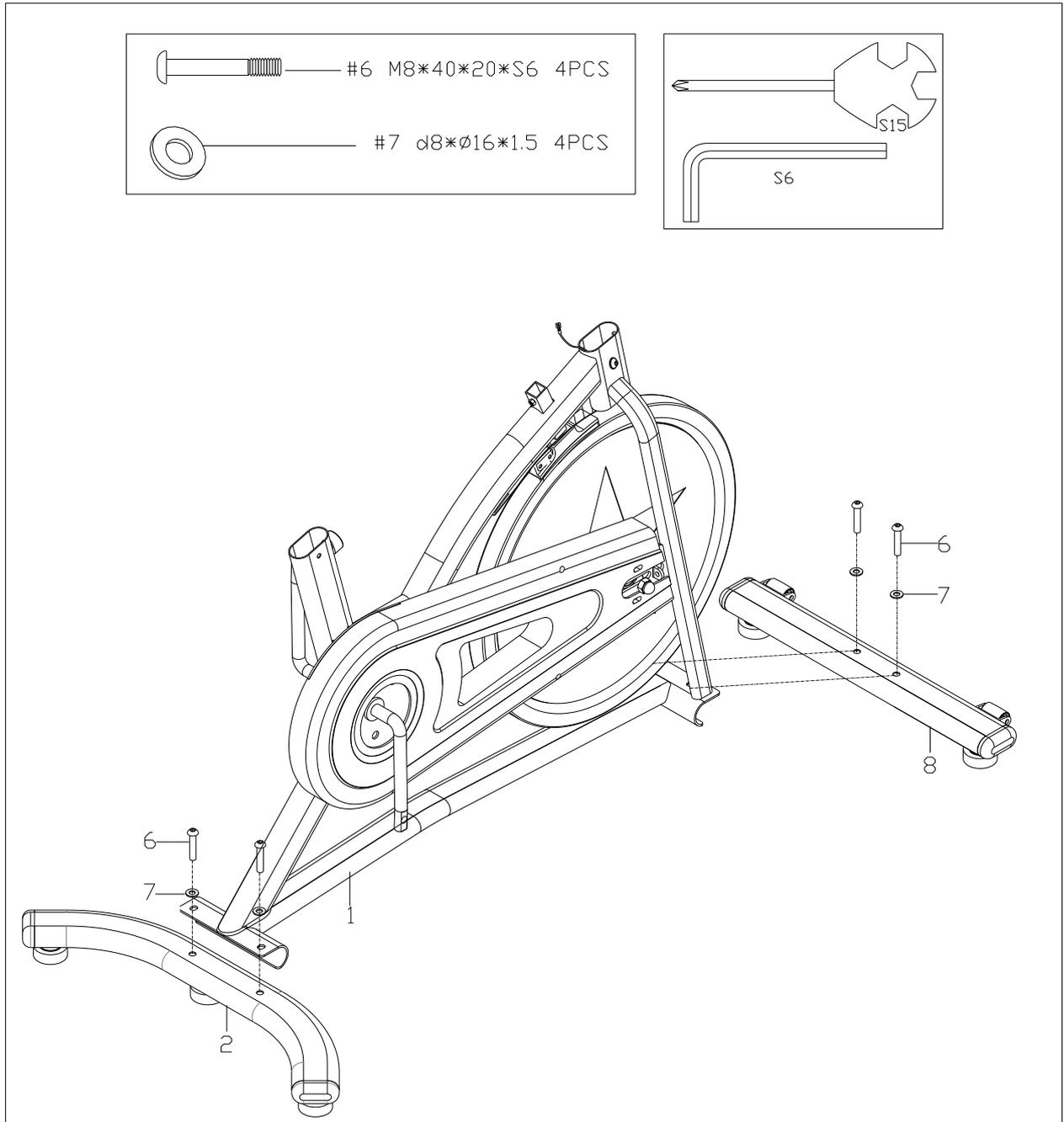
Fix the Front stabilizer (8) and the Rear stabilizer (2) onto the Main frame (1) with Screws (6) and Washers (7).
