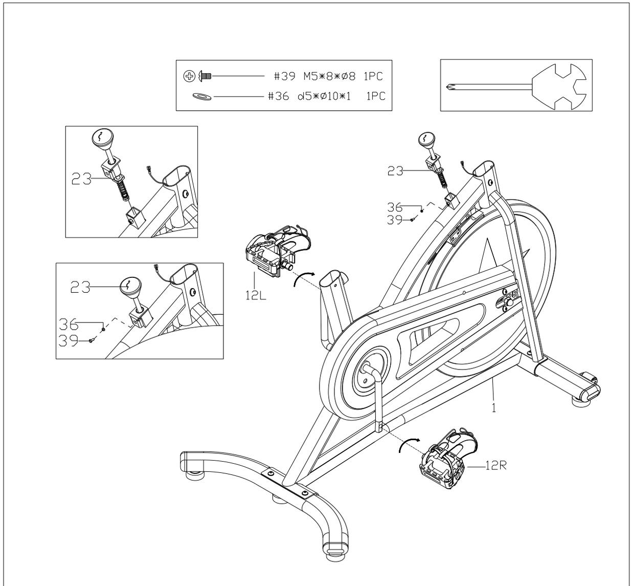
A. Push the Brake handle (23) into the Main frame (1) down slowly and then fix it with the Screw (39) and Washer (36).
