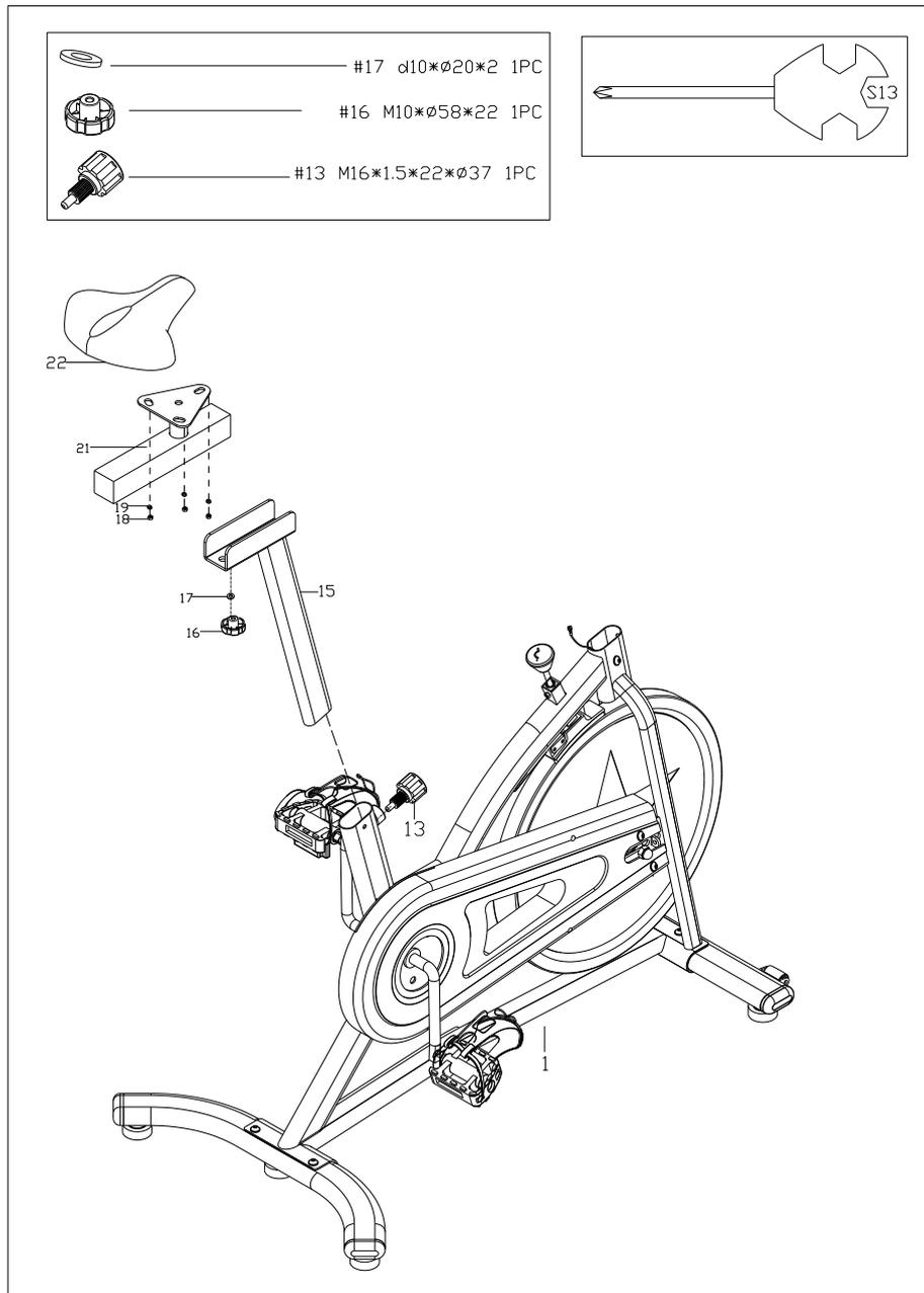
A. Fix the Saddle (22) onto the Saddle tube (21) with Washers (19) and Nylon nuts (18).
