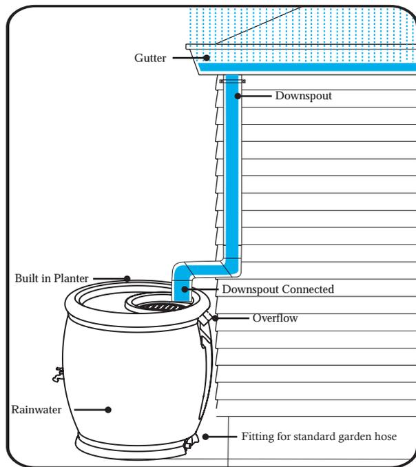
The Algreen Rain Barrel system is an easy way to collect and store natural rainwater.
