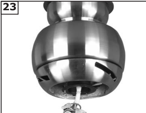
23 Lift fan to mounting bracket, aligning the "L" shape holes with the screws on the mounting bracket. Turn the fan clockwise to lock in position. Install the other two screws and tighten securely.
