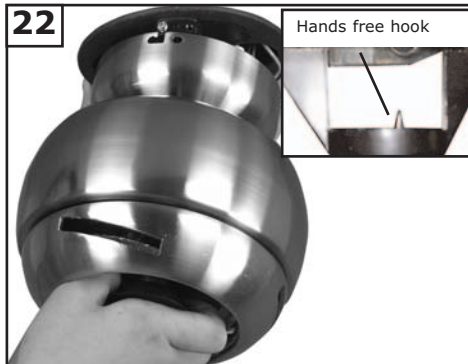
22 Hang fan from mounting bracket by the hands free hook into a closed hole on the edge of the Canopy. Note: For Canadian mounting refer to Step #10.
