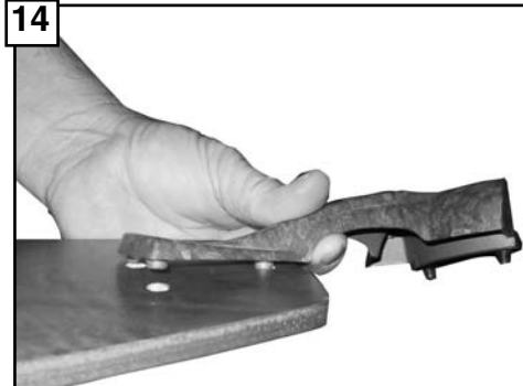
Place blade onto blade holder.
