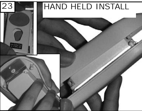
23 HAND HELD INSTALL Place face plate over battery compartment and buttons. Place remote over 2 pins on front cover. Attach cover of remote by placing over 4 pins and snapping into place.
