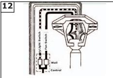
For control of fan and optional light from wall location, follow diagram above. NOTE: A professional electrician is recommended for this type of installation.
