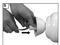
Thread wires and safety cable through downrod with canopy and yoke cover assembled.
