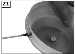
Remove the 3 screws from switch cap.
