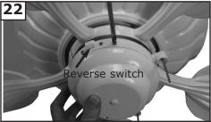
Install switch cap onto switch plate housing, align the 3 holes and install 3 screws and tighten securely. Setting the reverse switch in the left hand side will result in downward airflow and setting the switch in the right hand side will result in upward airflow.
