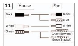
For pullchain controls, follow diagram above. Make sure that all exposed wiring is secured inside wire nuts. Note: Wires from house may vary in color and may not include ground wire. Are wiring is conplete, gently push wires into junction box with wire nuts pointing upward. Refer to point 3 of safety tips.
