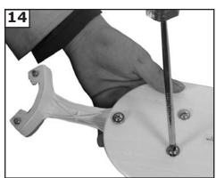
Install 3 screws and washers per blade and tighten securely. Repeat for all 5 blades
