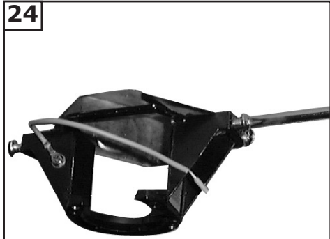
24 Take 4 screws from hardware pack and insert 2 one on each side of bracket to match the L slot screw holes in canopy. Keep 2 screws for later use.
