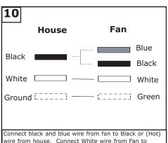
wire from house. Connect White wire from Fan to White (Neutral) wire from house. Connect Ground leads from mounting bracket and downrod to Ground lead from house. Refer to Safety Tips section of manual.
