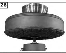
Lift fan to mounting bracket, aligning the "L" shape holes on the canopy with the screws on the mounting bracket. Turn the fan clockwise to lock in position. Re-install the screws removed in the previous step and tighten securely.
