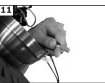
Make wire connections to power source using wire nuts provided. Make sure that no filiments are outside of the wirenut. After making the wire connections, the wires should be spread apart with the grounded conductor and the equipment-grounding conductor on one side of the outlet box and ungrounded conductor on the other side of the outlet box.
