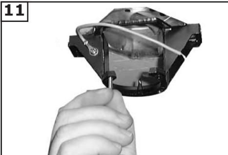
Make sure the studs protruding from the bottom of the Mounting bracket are installed with threads all the way through the bracket.
