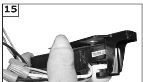
Slide remote receiver into mounting bracket.
