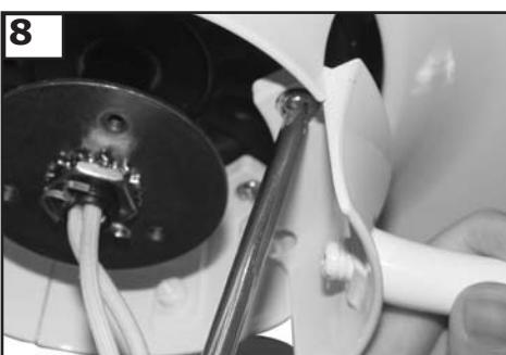
8 Remove 2 screws per blade holder. Remove blade holder. **When replacing blade holders make sure the screws are tightened securely to the motor.**
