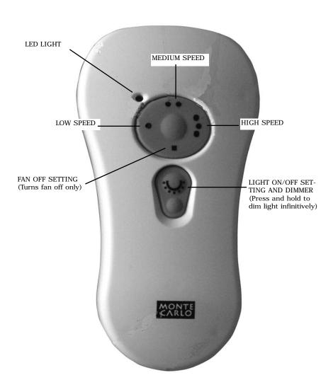
FAN SPEED Depress "I dot" for low speed, "2 dots" for medium or "3 dots" for high. To turn fan off press square".
