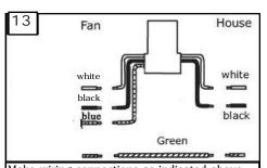
Make wiring connections as indicated above. White from fan to white from remote marked N. Blue from fan to blue from remote marked light. Black from fan to Black from remote marked L. White from house to white from remote marked AC N. Black from house to Black from remote marked AC L. Connect all green ground wires to Ground wire from House.
