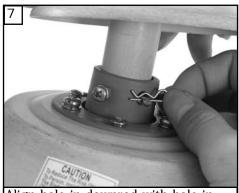
Align hole in downrod with hole in yoke and install cross pin. Install downrod into yoke. Install keeper into cross pin.
