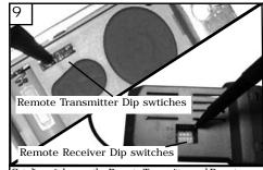
Set dip switches on the Remote Tiansmitter and Remote Receiver to the same settings. This must be done so the units will communcate properly. If you have other fans you can set to control from one transmitter by setting both receivers the same as the transmitter. If you have more than one fan with remote. You can set the dip switches to different positiosns to have seperate control.
