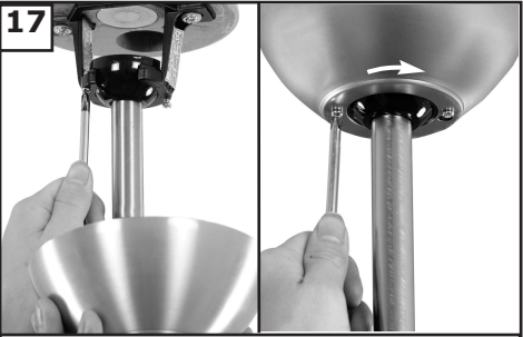
17 Loosen one and remove one preassembled screw from mounting bracket. Save screw. Lift canopy up, aligning its keyhole slot with the preassembled screw on mounting bracket and twist clockwise to lock in place. Re-install the removed screw and tighten all screws securely.
