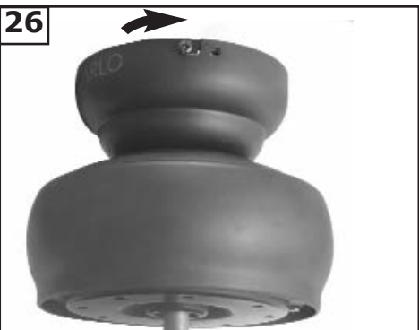
26 Lift fan to mounting bracket, aligning the "L" shape holes with the screws on the mounting bracket. Turn the fan clockwise to lock in position. Install the screws that were not installed from earlier step. Tighten securely.
