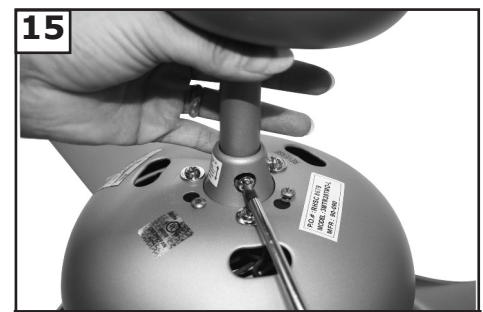
15 Place the downrod into the yoke aligning the holes on downrod with the holes on the yoke and then re-install the cross pin removed in step 12. Tighten securely.
