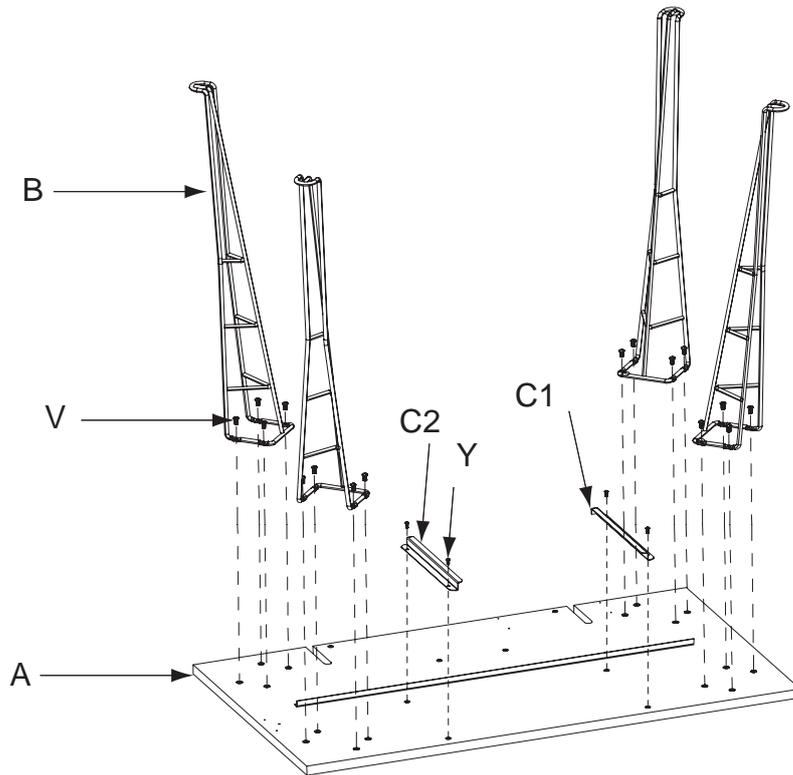
1. Fix the legs (B) to top panel (A) with screws (V), fix the drawer rail (C1 & C2) of drawer to top panel with screws (Y).
