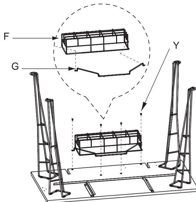
2. Insert the holding wire (G) into surge protector (F), then fix it with screws (Y).
