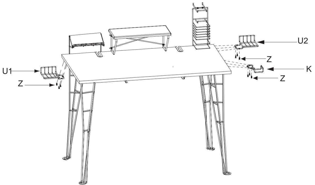
4. Fix the speaker tray (U1 & U2) to the top panel with screws (Z), fix the headphone holder (K) with screws (Z).
