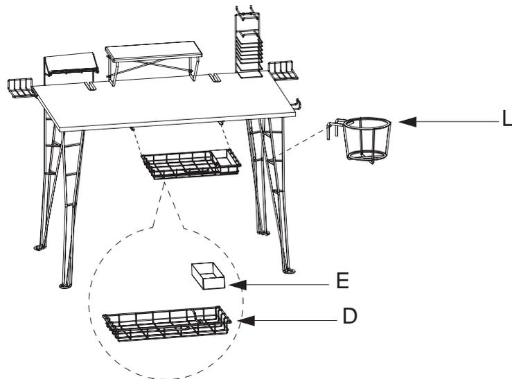
5. Fold the plastic sheet (E) to rectangular shape, then put it into drawer (D), insert the drawer into the rail, hang the cup hold (L) to the leg.
