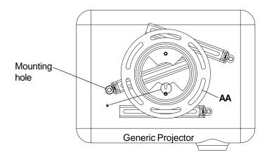
Attach adapter plate (AA) to projector using one screw (BB, CC, DD, or EE) for each channel as shown below. Tighten all screws, while keeping the center of gravity. Be sure that adapter plate (AA) is straight. Adjust the feet of the channels to keep the adapter plate level. Tighten all screws with 4 mm security allen wrench (FF), while keeping the center of gravity. If M3 screws are used, tighten using 2 mm security allen wrench (GG).
