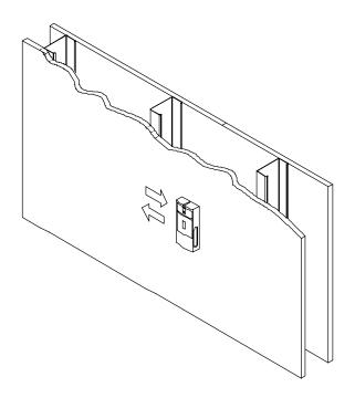
Use wall plate (A) as a template to mark slot centers on stud centers.
