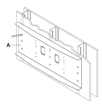
Drill twelve 3/4" (19 mm) dia. holes through drywall and studs. Insert togglers (**D**) as shown below.
