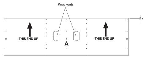
\*Note: The mounting hole which is closest to the lip of the plate indicates the up position.
