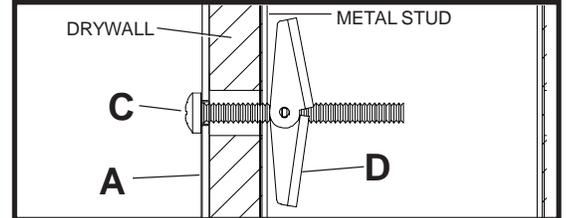
Pull screw (C) back until toggler (D) is flush with metal stud and hold. Thread screw through with fingers and loosely tighten.
