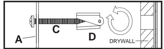
Place screw (C) through metal stud wall plate (A). Partially fasten toggler (D) to back of screw. Pivot toggler ends 90° and push through hole in drywall.
