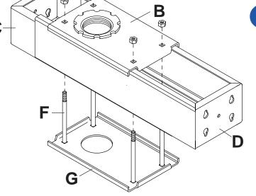
**IMPORTANT:** If installer is working above the ceiling, such as in an attic space, assemble exactly as pictured. If installer is working below the ceiling, reverse positions of carriage bolts (F) and nylock nuts (E).
