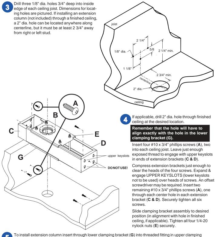
bracket (**B**). Tighten four or five complete turns until securely tight.
