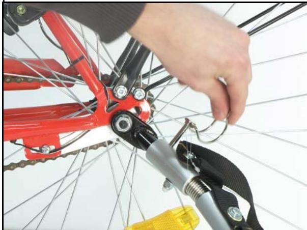
Push the safety pin through the hole and lock the safety pin.
