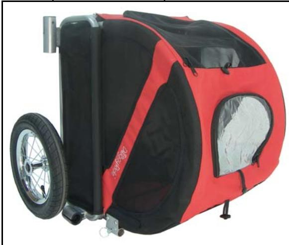
Install the tow bar into the holder on the centre on the front of the trailer. Use the quick release pin to secure the tow bar. The quick release pin is secured by a lever.
