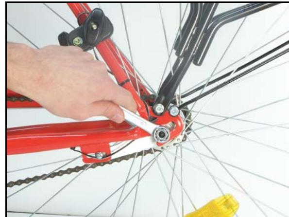
Place the hitch over the axle and position the pin facing backward. Screw the bolt again for the axle and lock it slightly.
