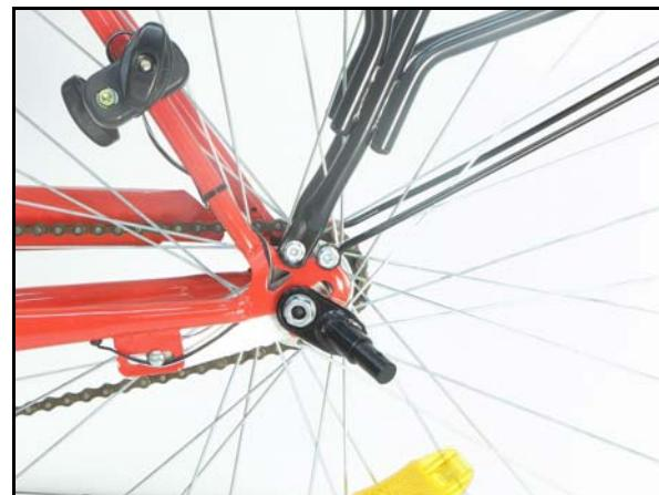
For correct positioning of the hitch to the trailer for a 28 or 26-inch bicycle ensure the right angle downward in such a way that the trailer is horizontally leveled behind the bicycle.
