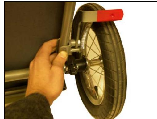
Insert the 2 bolts into the holes and secure the bolts. Use wrench no 10 to secure the parking brake bolts.
