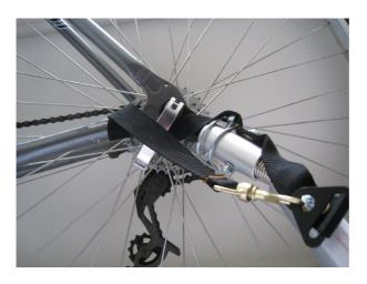
**Install Safety Flag**Join the pole section together. On the trailer's left side, insert the flag pole into the flag receptacle. (see image.)
