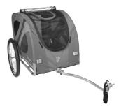
Once you have assembled the crate you can now assemble the trailer. Add the two wheels and the tow bar to the cabin to make a trailer.
