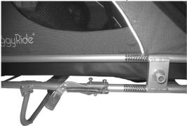
Install it using wrench #10 and a Phillips screwdriver. Unlock it before replacing the wheel on the stroller. The stroller is now ready for use. Always use the parking brake when leaving the stroller unattended, as only the left is locked and the stroller might turn when leaving it unattended.
