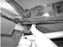
Once the cross bar is in the position push the detent pin back into the hole. The cabin is now ready to use as foldable crate or car carrier.
