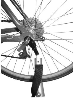
Hitch installation for bolted axles
