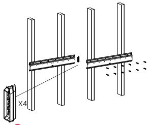
Slide Connector/End cap into mounted rail and repeat installation for second rail.
