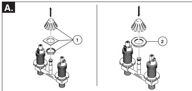
Remove plastic umbrella, spout nut and washer (1). Replace with thin nut (2) and plastic umbrella.
