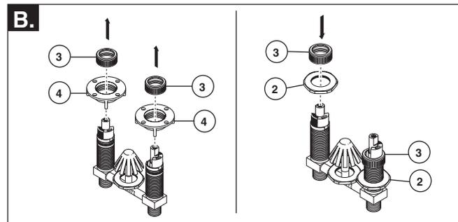
Remove two bonnet nuts (3). Remove two locknuts (4), and replace with thin nuts (2). Reinstall bonnet nuts (3).
