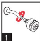
Remove existing shower head from shower arm. Remove any excess materials left on the threads of the shower arm.
