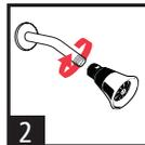
Hand tighten (no pliers needed) new head to shower arm. Plumber tape recommended to prevent leakage. Do not use plumber's putty.
