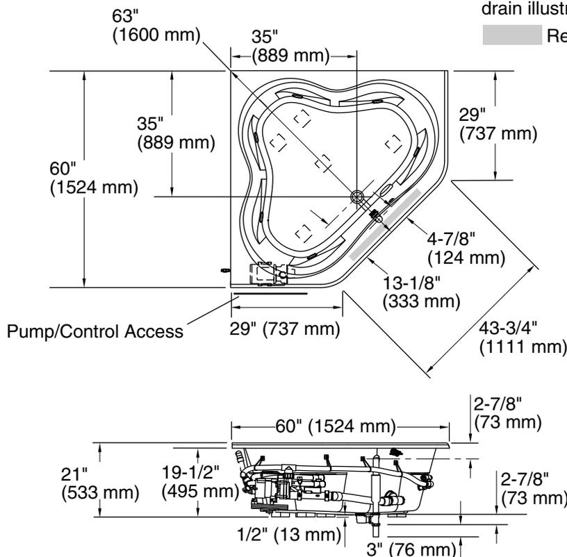
No change in measurements if connected with drain illustrated. (K-11677 or K-11677M)
