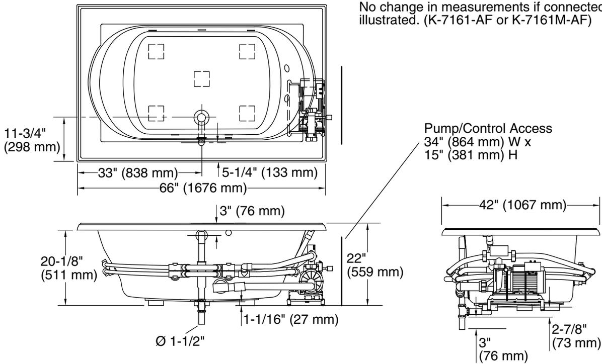
No change in measurements if connected with drain illustrated. (K-7161-AF or K-7161M-AF)
