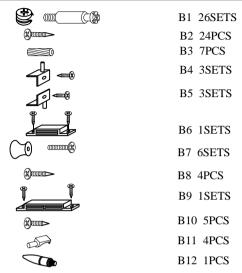
Apply a little glue B12 into the wood dowel holes when inserting wood dowels.
