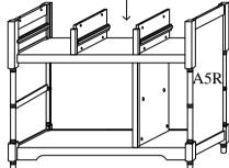
Insert the back panel A16 into the grooves of side panels A5(R&L) and bottom panel A4.
