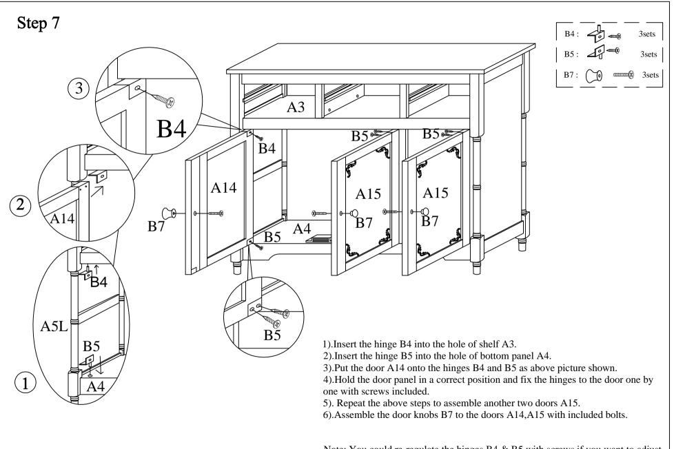
Note: You could re-regulate the hinges B4 & B5 with screws if you want to adjust the door gap.
