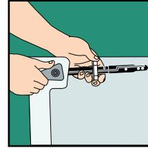
4. Unthread nut from new handle (reverse thread – turn opposite usual direction) and remove. Slide new lever through tank hole until handle shank fits snugly. Slip locknut over lever (flat side facing handle). Start nut on threads (reverse thread), but **DO NOT TIGHTEN FULLY.**
