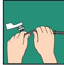
2. Continue to Step #3 for standard front-mount tank. **FOR SIDE OR ANGLE-MOUNT TANK, slowly** bend new lever arm to match old lever arm. Or, position new lever in tank to determine arm angle needed. Remove, then *slowly* bend new lever arm to match the angle of the tank. **DO NOT BEND ARM TOO QUICKLY OR BACK AND FORTH REPEATEDLY.**
