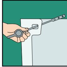
1. Remove tank lid. Disconnect the flapper chain/linkage from the lever. Unthread nut from old lever. Remove lever from tank.
