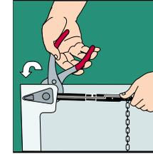
5. Connect flapper chain/linkage to hole in tank lever arm that provides the best lift. Chain should have slight slack when flapper is in the closed position. Replace lid and check lift action for proper flush. Tighten tank lever nut securely (**DO NOT OVERTIGHTEN**).
