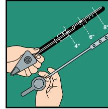
3. Measure length of existing lever (it should be 4", 6", 8" or 9"). If necessary, trim new lever at the cut line that matches the length of the old lever (hacksaw recommended for best results).
