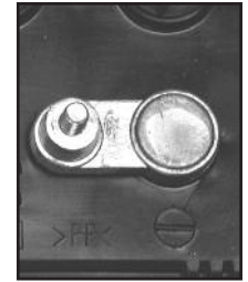
NEGATIVE POST HAS SMALLER DIAMETER
