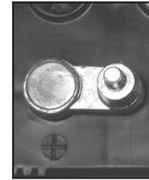
POSITIVE POST HAS LARGER DIAMETER
