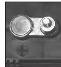
POSITIVE POST HAS LARGER DIAMETER
