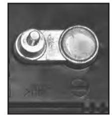
NEGATIVE POST HAS SMALLER DIAMETER
