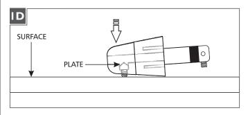
**5** Tap the conical connector on a hard surface with the set screw facing down, so the plate inside drops into place.
