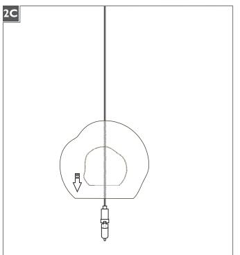
3 Lower the glass shade onto the socket assembly.
