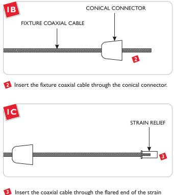
Insert the coaxial cable through the flared end of the strain relief.
