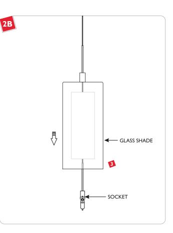
3 Lower the glass shade onto the socket assembly.
