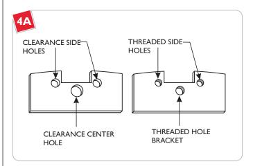
There are four mounting brackets, two with threaded holes and two with clearance holes. Each set uses a threaded and clearance hole bracket.
