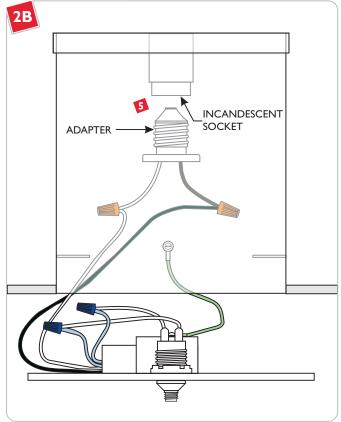
Screw the adapter tightly into the incandescent socket.
