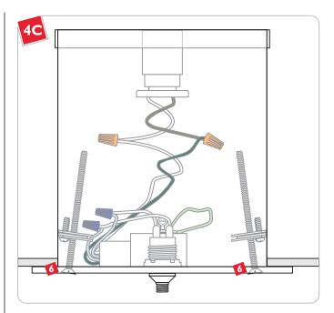
Screw the long #10-24 screws into the center hole of brackets.
