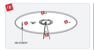
Secure the mounting plate to the anchors with the provided #8 screws.
