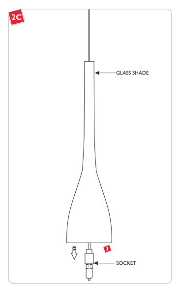
1 Lower the glass shade onto the socket assembly.
