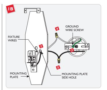
2 Feed the fixture wires through the mounting plate side hole.
