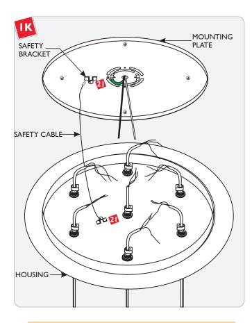
**NOTE:** It is recommended that one person holds the canopy while the electrician finishes the installation.
