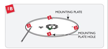
Align the mounting plate holes with the electrical box holes and mark four points onto the ceiling through the mounting holes.
