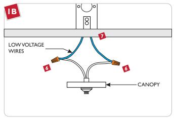
6 Connect each canopy wire to a low voltage wire with a wire nut.
