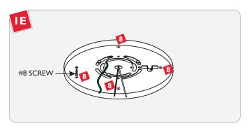
Secure the mounting plate to the four anchors with the four provided #8 screws.
