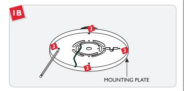
Align the mounting plate slots with the electrical box holes and mark four points onto the ceiling through the mounting holes.
