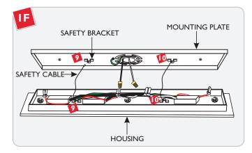
Insert one end of the safety cable into the mounting plate safety bracket and insert the other end into the housing safety bracket.
