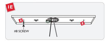
Secure the mounting plate to the anchors with the provided #8 screws.
