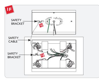
Insert one end of the safety cable into the mounting plate safety bracket and insert the other end into the housing safety bracket.
