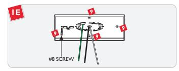
Secure the mounting plate to the anchors with the provided #8 screws.
