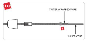
Slide the outer wrapped wire back to expose the inner wire.
