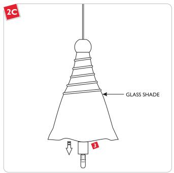
13 Lower the glass shade onto the socket assembly.
