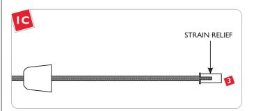
3 Insert the coaxial cable through the flared end of the strain relief.
